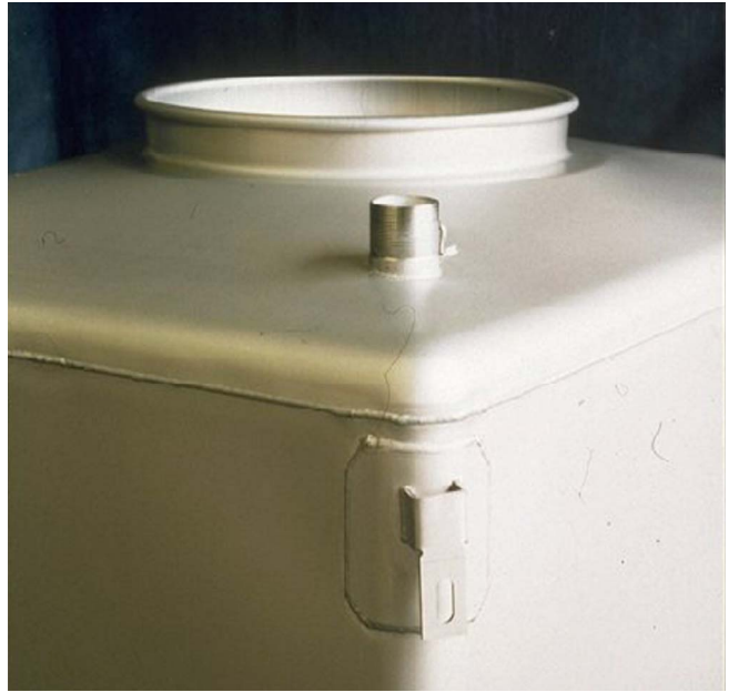
Figure 7. The same stainless steel tank after pickling. Acid pickling effectively removes heat tint and other surface contamination which results from fabrication, such as embedded iron and rust.
