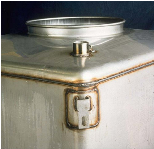
Figure 6. A stainless steel tank before pickling.
