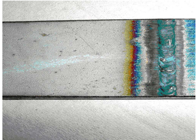
Figure 3. Heat tints (weld discolouration) on the root of a stainless steel butt weld (TIG/GTAW with argon gas purging) of 3 mm thick UNS S31603 (steel number 1.4404, Type 316L) pipe (300 mm ID).
