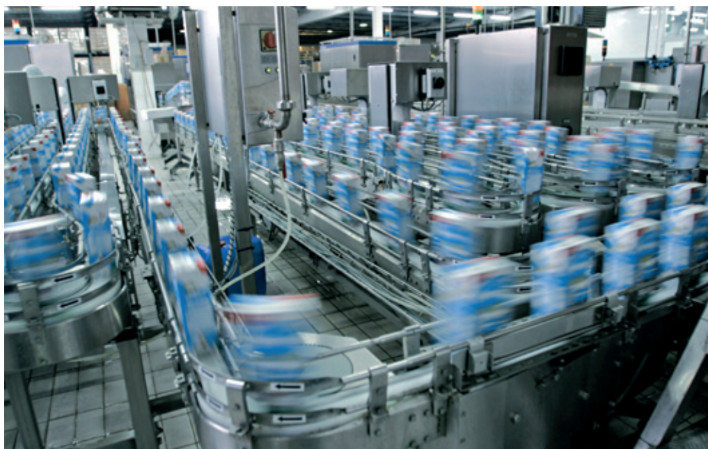
Lactic acid is quite aggressive and requires corrosion-resistant materials like stainless steel.
