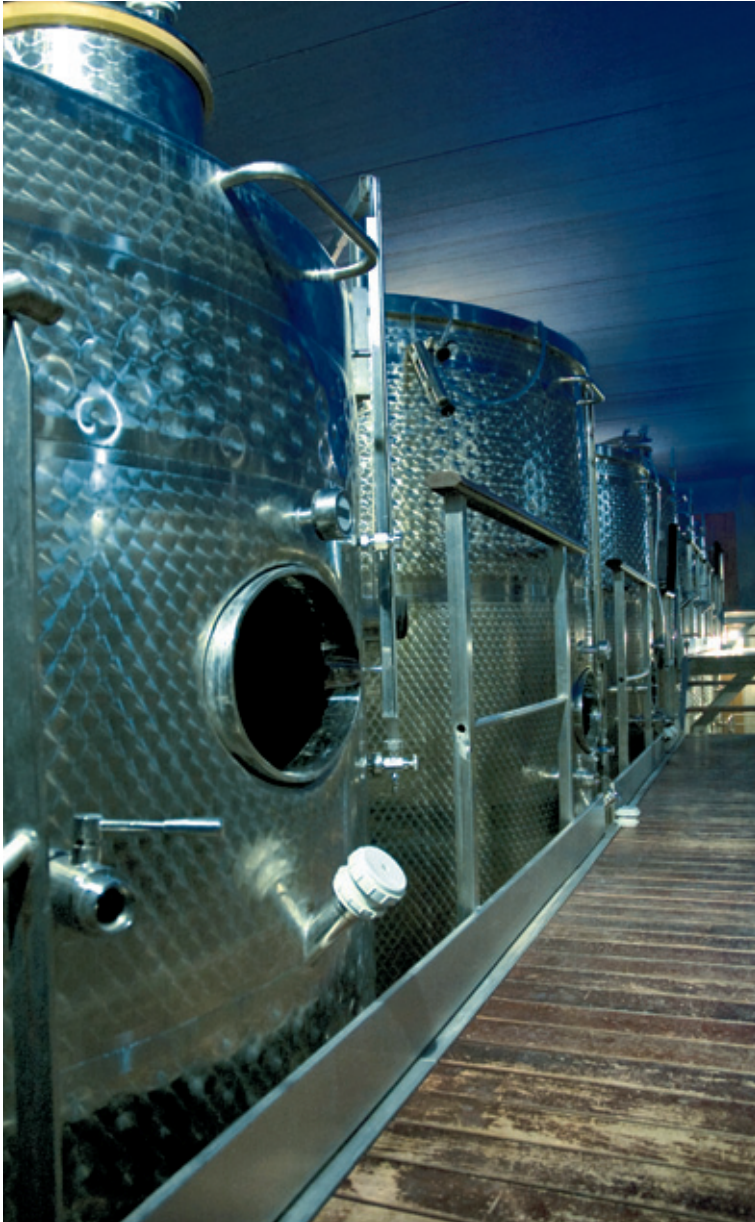
Stainless steel resists the acidic conditions typically found in wine tanks.
